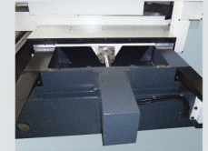
■ Z Axis Square Way Design / Z Axis Ball Screw Mounted at Central Slide Z軸方軌設計 / Z軸滾珠導螺桿於軌道中央設計
