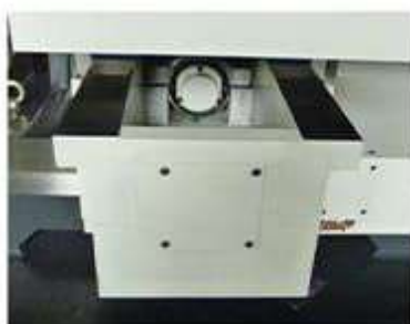
X/Z軸方軌設計 / Z軸滾珠導螺桿於軌道中央設計 X/Z Axis Square Way Design / Z Axis Ball Screw Mounted at Central Slide
