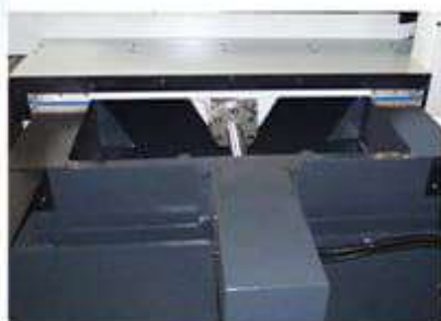
X/Z軸方軌設計 / Z軸滾珠導螺桿於軌道中央設計 X/Z Axis Square Way Design / Z Axis Ball Screw Mounted at Central Slide
